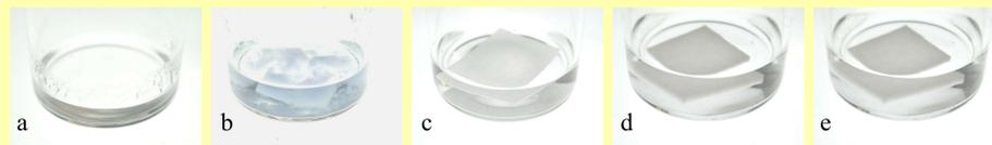
Fig. 2: Cellulose membranes in neat TFA after 24 h: a) Starting cellulose membrane; b) " $\beta$ -Ala" membrane; c) AC-S membrane (0.4  $\mu\text{mol}/\text{cm}^2$ ); d) AC-L membrane (2  $\mu\text{mol}/\text{cm}^2$ ); e) AC-X membrane (5  $\mu\text{mol}/\text{cm}^2$ ).
