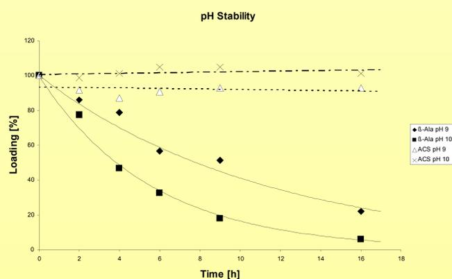
Fig.1: Hydrolysis of AC-S and  $\beta$ -alanine modified membranes (starting functionality set to 100%)
