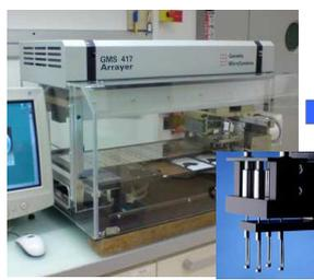
Printing on specially prepared<sup>(4)</sup> glass slides with 500 µm pin
