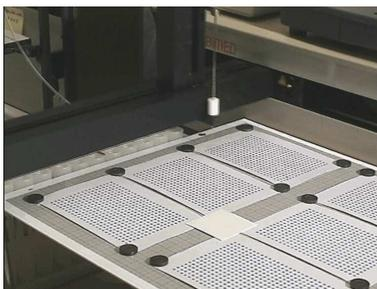
Parallel SPOT-synthesis on a cellulose membrane
